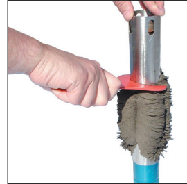
Cleaning the core using the supplied cleaning tool & core cleaning post (optional).
